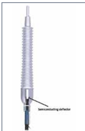
Fig. 1: Schematic of flexible dry-type outdoor termination.
